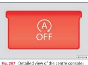
Fig. 207 Detailed view of the centre console Start-Stop function button
