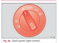
Turn the switch to the required position >>> Fig. 40.
