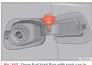
Fig. 237 Open fuel tank flap with tank cap in the holder
