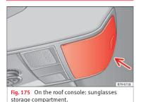
To *open*, press and release the button **>>> Fig. 175** (arrow).
