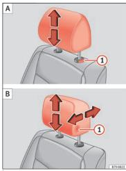
Fig. 150 A: Adjust the head restraints with no possibility of lengthways direction adjustment; B: Adjust the head restraints with lengthways direction adjustment
