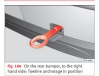
The location for the removable towline anchorage is on the right-hand side of the rear bumper **»** Fig. 104. For vehicles with a factory fitted towing bracket, there is **no** fitting behind the cover to insert the towline anchorage. For towing, fit and use the tow hitch **»** page 235, **» 0**.
