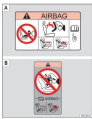
**Fig. 34** Airbag stickers - version 1: on the passenger-side sun blind **A** and on the rear frame of the front passenger's door **B**.
