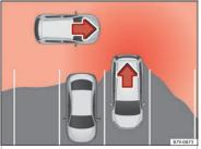
**Fig. 226** Schematic representation of the rear cross traffic alert: zone monitored around the vehicle exiting the parking space.
