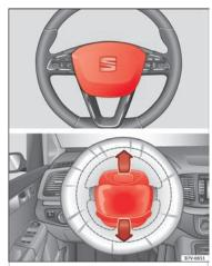
Fig. 25 Location and deployment area of the front airbag for the driver
