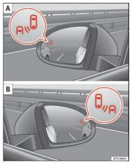
**Fig. 222** In the exterior mirrors: indication of the blind spot detector.
