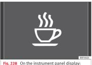
**Fig. 228** On the instrument panel display: tiredness detection symbol
