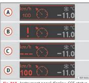
Fig. 219 Instrument panel display: CCS status indications.
