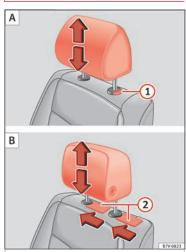
Fig. 152 A: Fitting the head restraints with no possibility of lengthways direction adjustment; B: Fitting the head restraints with lengthways direction adjustment
