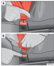
Fig. 87 Insert the latch plate into the buckle
