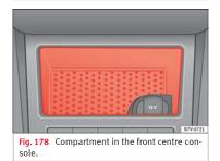
There is an open compartment on the centre console **»** Fig. 178 in which there may be a 12 volt power socket **»** page 170.
