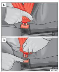
Fig. 21 Positioning and removing the seat belt buckle.
