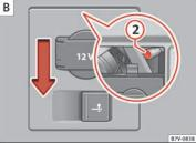
Fig. 113 On the side of the luggage compartment: removing the left and right hand side rear lights. (1) remove the cap; (2) attachment screw
