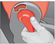
Fig. 160 Unlocking the folding backrest of the front passenger seat
