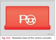
Fig. 213 Detailed view of the centre console button to switch the park assist system on manually
