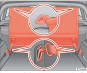
Fig. 167 In the luggage compartment: install the net partition behind the second row of seats.
